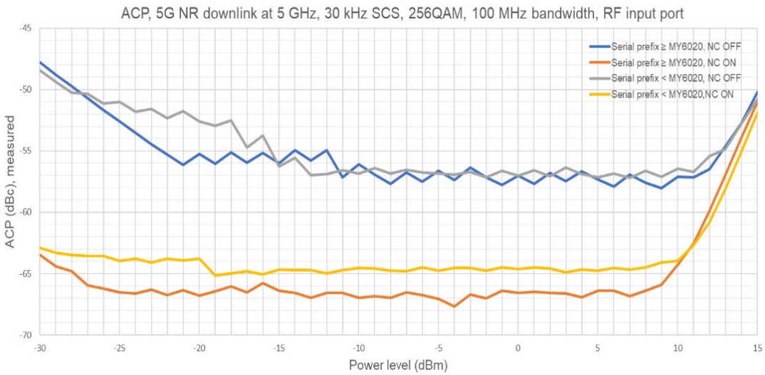
Figure 13. 5G NR downlink ACP vs. input power level at 5 GHz with 100 MHz bandwidth, 30 kHz SCS, 256 QAM
